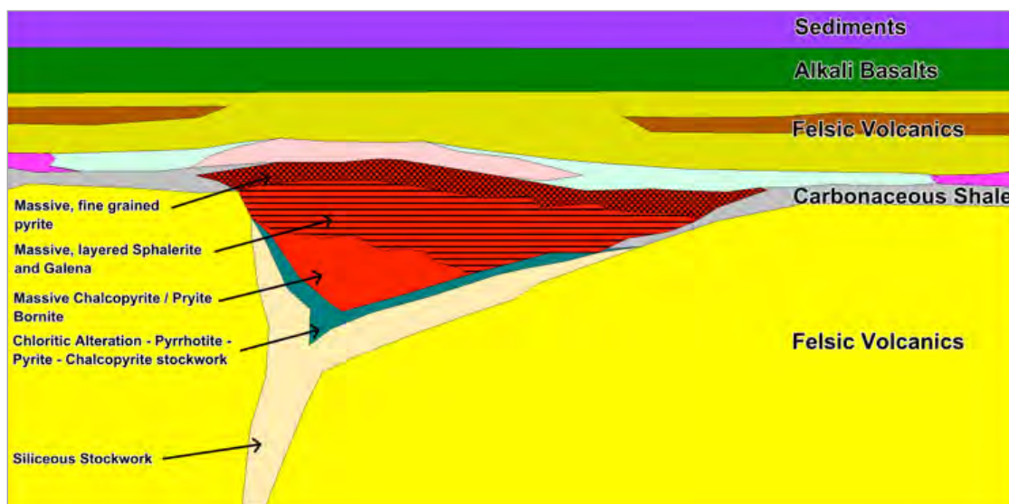
Figure 9: Schematic section through a VMS Zn/Pb/Cu deposit (model)
