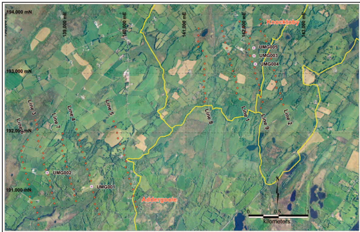
Figure 10: Induced Polarisation Survey and Drillhole Location Map
