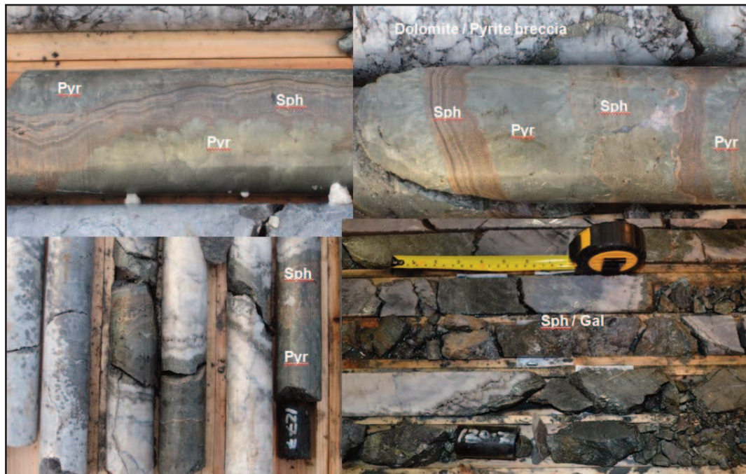
Figure 19: Photographs of high grade mineralisation from UMK-001 (Pyr - Pyrite, Sph - Sphalerite, Gal -Galena)
