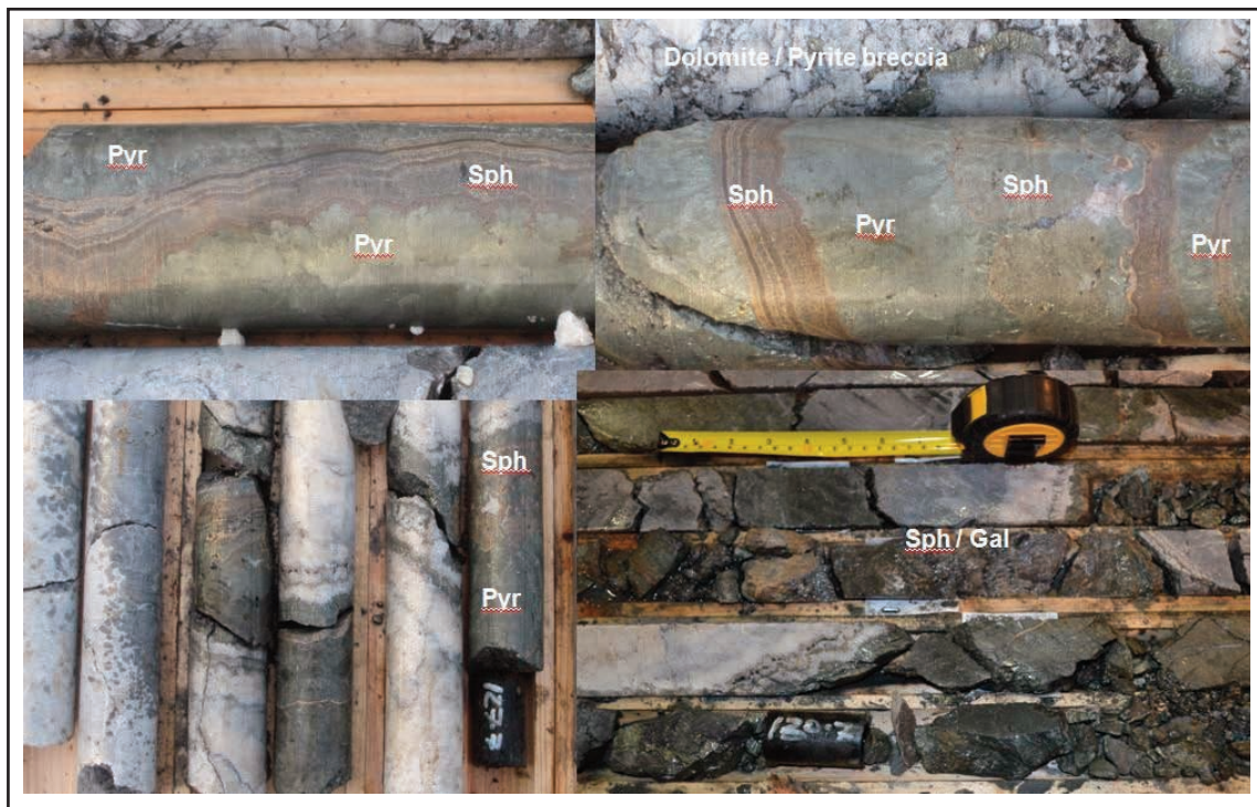
Figure 14: Photographs of high grade mineralisation from Kinnity (drillhole UMK-001: Pyr - Pyrite, Sph - Sphalerite, Gal - Galena)
